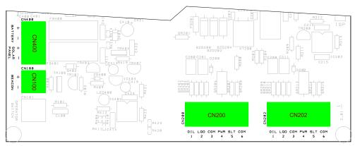
Figure 2 - Solar panel, battery and probe terminal locations
